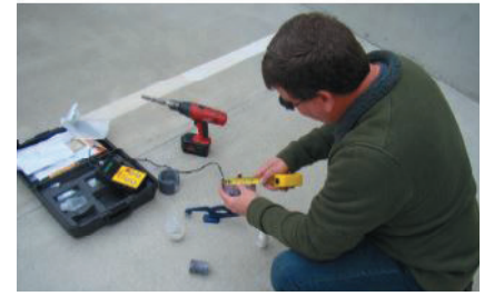
Figure 7 Chloride Ion & Carbonation Testing
